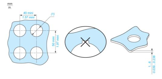
(1) Ø30.75 mm recommended (Ø30.5 mm  $_0^{+0.5}$ ) / Ø1.21 in. recommended (Ø1.20 in.  $_0^{+0.019}$ )
