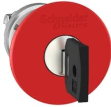
Head for emergency switching off push button, Harmony XB4, red 40mm stop, 22mm trigger and latching key release, key 3131A
