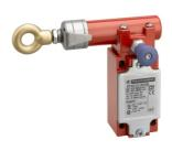
Latching emergency stop rope pull switch, Telemecanique rope pull switches XY2C, e XY2CJ, left side, 1NC+1 NO, Pg13.5
