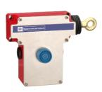
Latching emergency stop rope pull switch, Telemecanique rope pull switches XY2C, e XY2CE, RH side -1NC+1 NO, booted pushbutton
