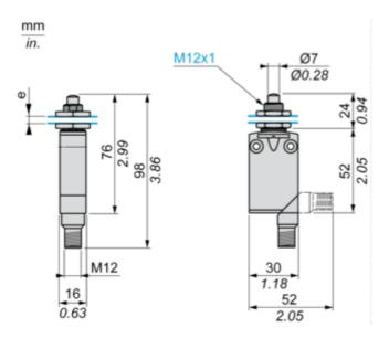
$\mathbf{e}$  : 8 mm max, panel cut-out Ø 12.5 mm, fixing nut thickness 3.5 mm.
