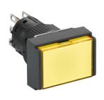
Illuminated monolithic push button, Harmony XB6E, rectangle yellow illumin pushbutton Ø 16 flush pushtorelease 12 VDCpolarised 1CO
