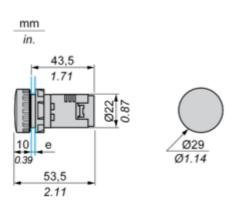
e: clamping thickness: 1 mm to 6 mm / 0.03 in. to 0.24 in.
