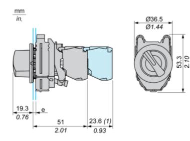
e : clamping thickness: 1 to 6 mm / 0.04 to 0.24 in.(1) : Additional row of contacts
