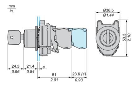
$\boldsymbol{e}$  : clamping thickness: 1 to 6 mm / 0.04 to 0.24 in. (1) : Additional row of contacts
