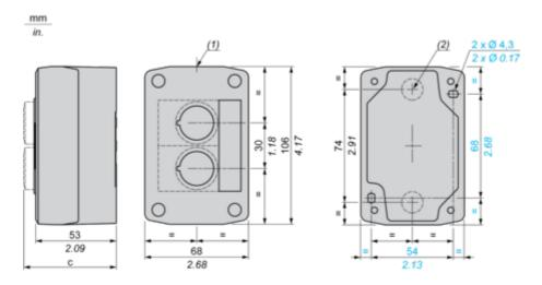
(1) 2 knock-outs for Pg 13.5 cable gland, maximum capacity 12 mm/0.47 in.(2) Knock-out for cable entry, maximum capacity 14 mm/0.55 in.
