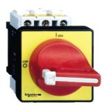
Switch disconnector,TeSys Control,for ON/emergency stop,32A, 4 screws fixing,for mounting on door
