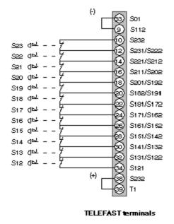
NOTE: If less than 12 contacts are being used, the input terminals that are not in use must be bridged.
