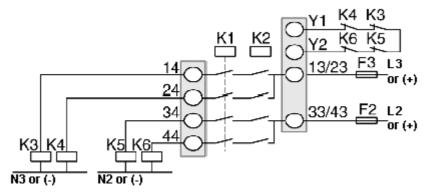
Connection of the Safety System Reactivation Function
