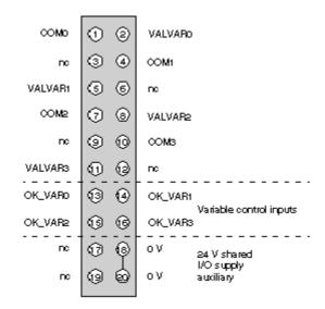
COMx - VALVARx: potential free contact to validate variable speed controller
