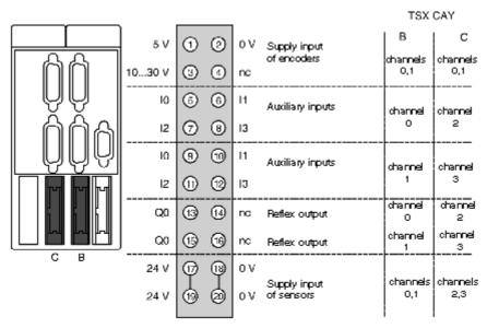
TSX CAY 2• module: Channels 0 and 1 TSX CAY 4• module: Channels 0,1,2 and 3 TSX CAY 33• module: Channels 0,1 and 2
