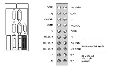
COMx – VALVARx: potential free contact to validate variable speed controller OK\_VARx: variable speed controller input check
