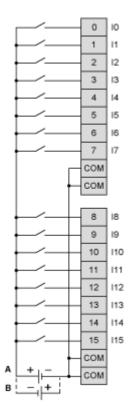
The 4 COM terminals are connected internally
