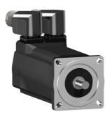
servo motor SH3 070, 2,04Nm,key,multi, brake, 90°conn, IP65, IP67, 8k RPM
