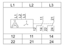
L1,L2,L3 : Supply to be monitored 11-14,12 : 1st C/O contact of output relay 21-24,22 : 2nd C/O contact of output relay **Technical Description**
