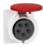
Socket, Mureva PK, panel-mounted, fast connection, 32A, 3P+N+E, 400V, IP44
