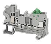
Terminal block, Linergy TR, hybrid, feed through, 2 points, screw-IDC, 2.5mm², grey
