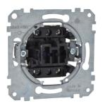
Switch, Merten inserts, mechanism, 3-pole 1-way, 16AX, screw terminals, IP20,
