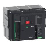
Circuit breaker frame, MasterPact MTZ2 16H1 drawout for MicroLogic X, 1600A, 66kA/415VAC (Icu), 3P
