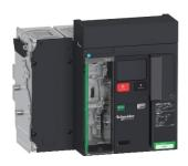
Circuit breaker frame, MasterPact MTZ1 16H2 drawout for MicroLogic X, 1600A, 50kA/415VAC (Icu), 4P
