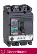
Circuit breaker, ComPact NSX100HB1, 75kA/690VAC, MicroLogic 2.2M trip unit 100A, 3 poles 3d
