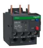
Thermal overload relay, TeSys Deca, 690VAC, 23 to 32A, 1NO+1NC, class 10A, for D25…D38, for unbalanced loads
