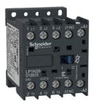
Contactor, TeSys K, 3P, AC-3/ AC-3e, 440V, 9A, 1NC aux, 24V DC coil,with integral suppression device
