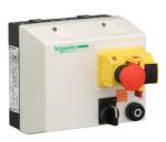
Enclosed reversing starter,TeSys LG,1-1.6A,380/400V AC coil,including 2 LC1K,GV2ME,pushbutton,2-pos switch
