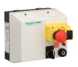
Enclosed reversing starter, TeSys LG,1-1.6A,220/230V AC coil, including 2 LC1K, GV2ME, pushbutton, 2-pos switch
