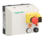
Enclosed DOL starter, TeSys LG, 2.5-4A,400V AC coil, including 1 LC1K, GV2ME with emergency stop, 2 pushbuttons
