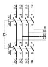
Electrical interlocking of reversers fitted with mechanical interlock without integral electrical contacts: LA9 F
