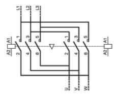
Reversing contactors for motor control LC2 F: 2xLC1 F Vertically mounted
