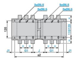
NOTE: Bar fixing centers Vertical: 120 mm, Horizontal: a2 see table.
