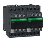
Changeover Contactor, TeSys Deca, 4P(4NO), AC-1, <= 440V 25A, 24V DC coil, screw clamp terminal
