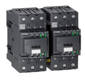
Reversing contactor, TeSys Deca, 3P(3NO), AC-3/AC-3e, <=440V, 66A, 24...60V AC/DC coil, EverLink BTR screws
