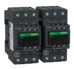
Reversing Contactor, TeSys Deca, 3P(3NO), AC-3, <=440V, 50A, 200V AC 50/60Hz coil, screw clamp terminals
