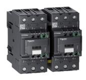
Reversing contactor, TeSys Deca, 3P(3NO), AC-3/AC-3e, <=440V, 50A, 24V DC coil, EverLink BTR screws
