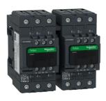
Reversing contactor, TeSys Deca, 3P(3NO), AC-3, <=440V, 40A, 440V AC 50/60Hz coil, screw clamp terminals
