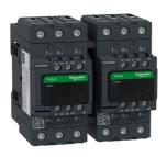
Reversing Contactor, TeSys Deca, 3P(3NO), AC-3, <=440V, 40A, 24V AC 50/60Hz coil, screw clamp terminals
