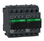
Reversing Contactor, TeSys Deca, 3P(3NO), AC-3, <=440V, 38A, 24V DC low consumption coil, screw clamp terminals
