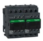
Reversing Contactor, TeSys Deca, 3P(3NO), AC-3, <=440V, 32A, 230V AC 50/60Hz coil, with mechanical and electrical interlocking, screw clamp terminals
