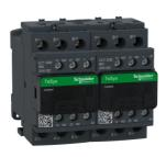
Reversing Contactor, TeSys Deca, 3P(3NO), AC-3, <=440V, 32A, 24V DC coil, with mechanical and electrical interlocking, screw clamp terminals
