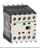
TeSys K contactor , 3P , AC-3 <= 440 V 12 A , 1 NO aux. , 48 V AC coil
