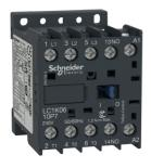
Contactor, TeSys K, 3P, AC-3/ AC-3e,<=440V 9A, aux. 1NO, 400...415V AC coil
