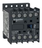
Contactor, TeSys K, 3P, AC-3/ AC-3e,440V 9A, 1NO aux, 220...230V AC coil, with integral suppression device
