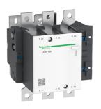
IEC contactor, TeSys F, nonreversing, 150A, 100HP at 480VAC, 3 phase, 3 pole, 3 NO, 120VAC 50/60Hz coil, open style
