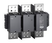
TeSys F contactor - 3P (3 NO) - AC-1 - <= 1000 V 1400 A - coil 265...277 V AC
