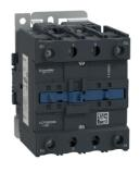
Contactor, TeSys Deca, 4P(2NO+2NC),AC-1, <=440V, 80 A 230V AC 50/60Hz coil, screw clamp terminal
