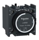
Time delay contact block,TeSys Deca,1NO+1NC,on-delay 1-30s,front,with 40±15ms switching time between NC opening and NO closing
