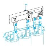
Feed unit for dry type transformers, Canalis KTC, copper, 3200A, 3L+PE, made to measure, neutral N5, white RAL9001
