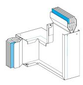
Edgewise and flat zed unit, Canalis KTC, copper, 1600A, 3L+PE, made to measure, neutral N1, white RAL9001
