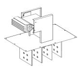
Flat elbow feed unit, Canalis KTC, copper, 1350A, 3L+PE, made to measure dimensions, neutral N4, white RAL9001
