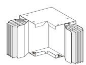
Flat elbow, Canalis KTA, aluminium, 3200A, 3L+N+PE, high Icw, N2, 1 made to measure short branch, right angle
