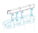
Feed unit for dry type transformers, Canalis KTA, aluminium, 3200A, 3L+N+PE, high Icw, made to measure, N2, RAL9001
